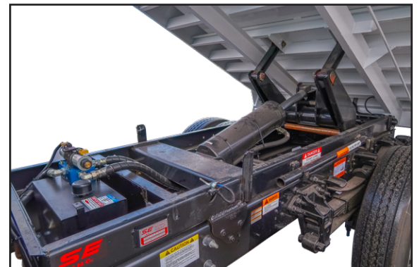
Dual manual-control Hoist Secure Locking Arms
